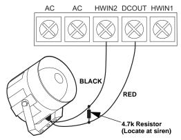
Figure 5. Hardwire Exterior Siren with Supervision
