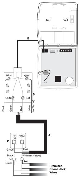
Figure 8. Full Line Seizure Wiring with an RJ-31X
