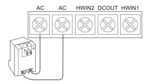
Figure 10. Connecting the Power Transformer
