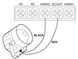
Figure 6. Hardwire Exterior Siren without Supervision
