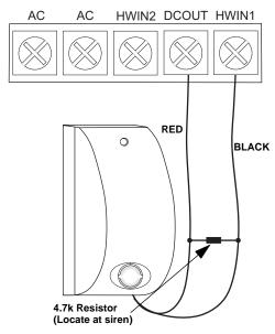
Figure 4. Hardwire Interior Siren with Supervision
