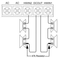
Figure 7. Connecting Normally Closed Hardwire Reed Switches
