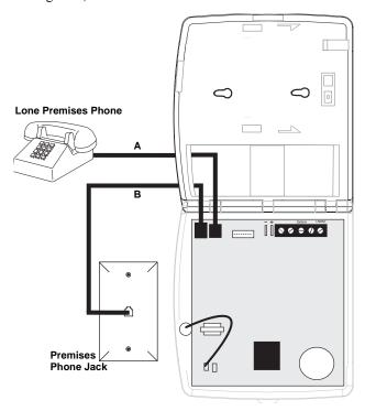
Figure 9. Full Line Seizure Wiring with 1 Premises
