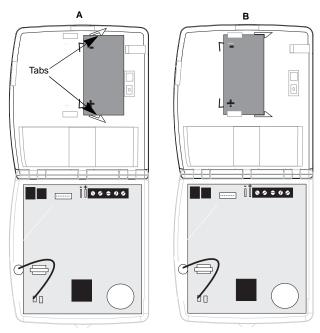
Figure 11.Installing the Panel Backup Battery
