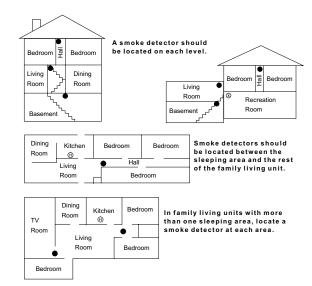
NOTE: Ceiling-mounted smoke detectors should be located in the center of the room or hall, or not less than 4 inches from the wall. When the detector is mounted on the wall, the top of the detector should be 4 to 12 inches from the ceiling.
