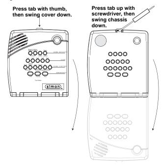
Figure 2. Opening the Panel Cover and Chassis
