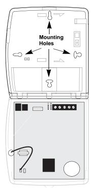
Figure 3. Panel Mounting Hole Locations
